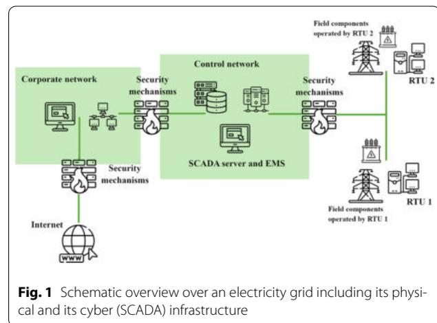
**Fig. 1** Schematic overview over an electricity grid including its physical and its cyber (SCADA) infrastructure
