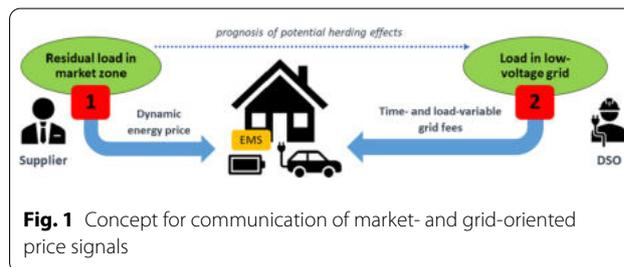
**Fig. 1** Concept for communication of market- and grid-oriented price signals
