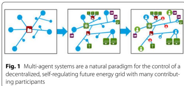
**Fig. 1** Multi-agent systems are a natural paradigm for the control of a decentralized, self-regulating future energy grid with many contributing participants
